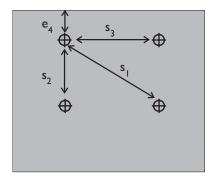
Anchor #4 is the most effected by edge and spacing conditions in the anchor group.
