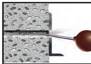
Blow out dust from the hole
