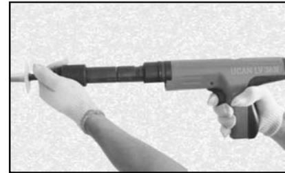
1. With the point out, insert fastener into the guide until it is held in place by the guide.
