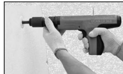
3. Insert the magazine into the base of the handgrip. Slide the magazine upwards until it is flush with the bottom of the grip. Always insert magazine from the bottom of the tool.
