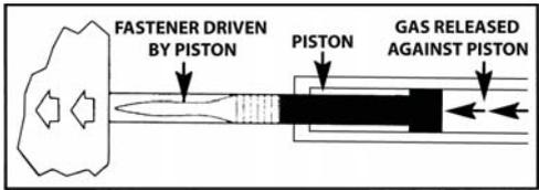
There are three velocity classes of powder actuated tools. The velocity class of the tool is determined by a ballistic test utilizing the lightest fastener and the strongest cartridge which is designated for use with the tool by the manufacturer.
